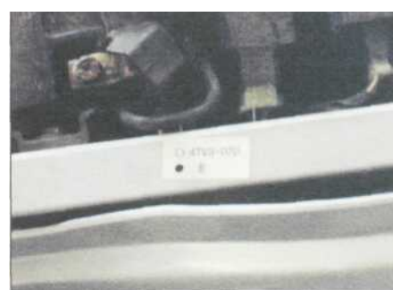
The model code label is on the top of the left-hand sub-frame spar under the seat
