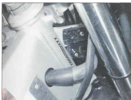
The frame number is stamped on the right-hand side of the steering head
