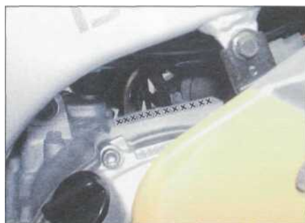
The engine number is stamped into the top of the crankcase on the right-hand side of the engine
