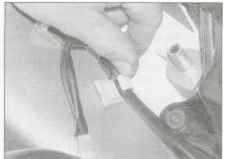
8.2 Release the sidelight wiring from its clip on the fairing
