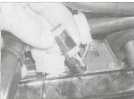
24.1c ... to access the diode
