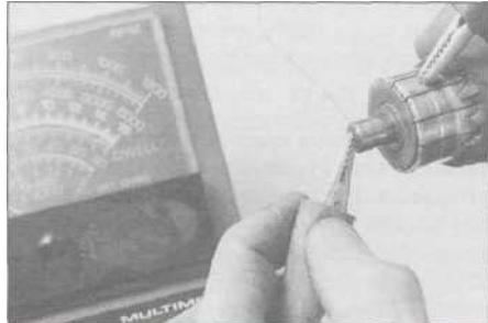
30.11 b There should be no continuity between the commutator bars and the armature shaft
