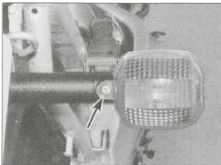
12.1 Remove the screw (arrowed) and detach the lens ...
