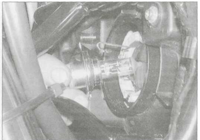
7.3b ... and remove the bulb
