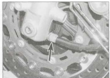
15.6 Unscrew the knurled ring (arrowed) and detach the cable ...
