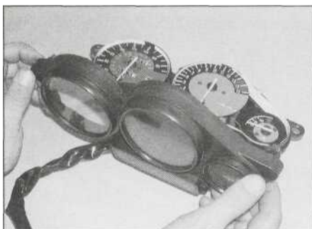
16.5b ... and lift off the front cover
