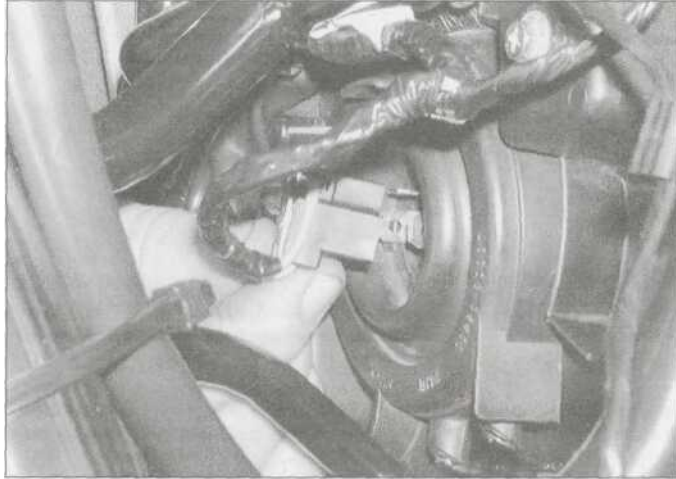
7.2a Disconnect the wiring connector...
