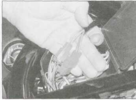
18.1b Ignition switch wiring connectors - FZS models
