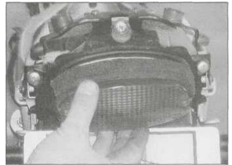
9.4 Make sure the lens sits properly on the rubber seal
