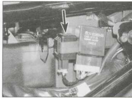
11.3b Turn signal relay (arrowed)- FZS models
