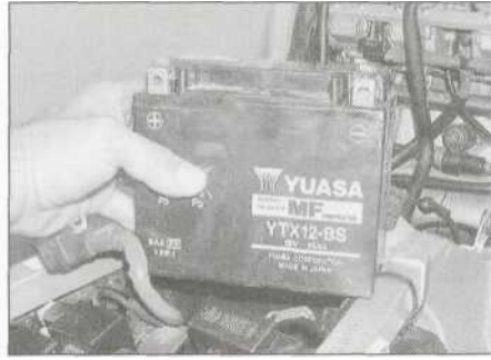
3.2c ... and remove the battery
