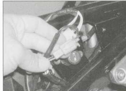
22.2b Sidestand switch wiring connector • FZS models
