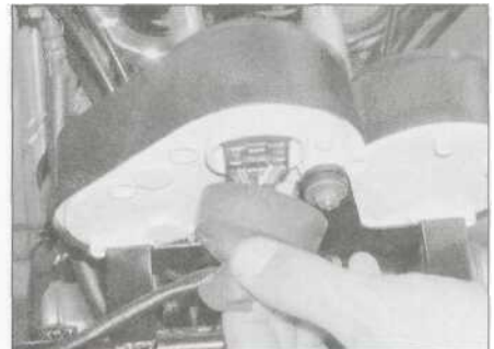
15.3a Pull back the rubber cover and disconnect the wiring connector
