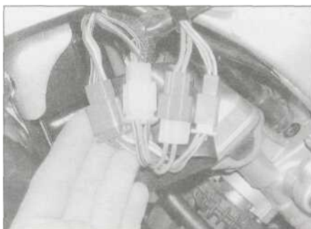
19.3a Left-hand switch wiring connectors - YZF models
