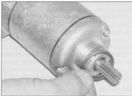
29.5 Fit a new O-ring into the groove
