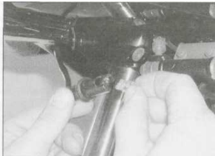
7.8b ... and carefully pull the bulb from the holder
