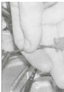
22.2a Sidestand switch wiring connector - YZF models
