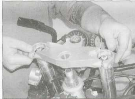
18.5c ... and ease the yoke up off the forks
