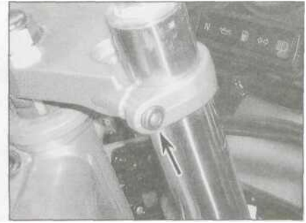
18.5a Slacken the fork clamp bolt (arrowed) on each side ...
