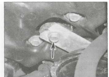
26.6 Horn mounting bolt (arrowed) • YZF models
