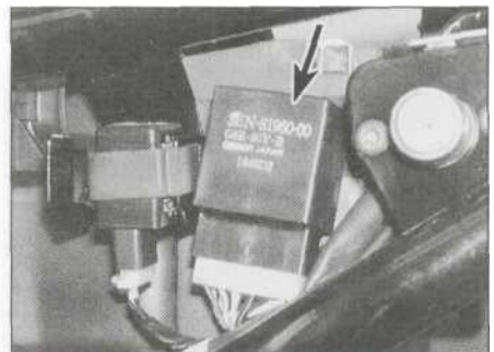
25.2b Starter circuit cut-off relay - FZS models
