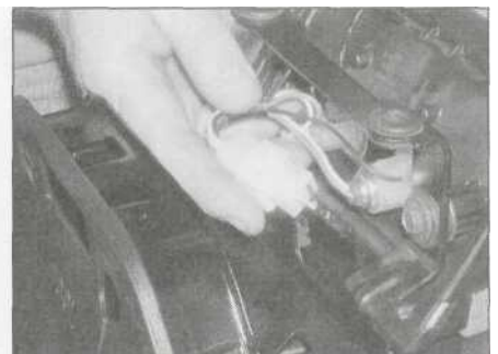
10.2 Disconnect the wiring connector
