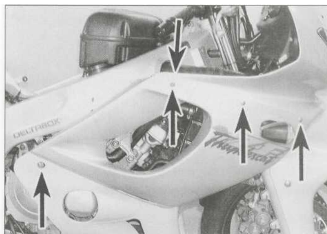
3.9a Remove the five screws (arrowed) securing the top and middle of the panel...
