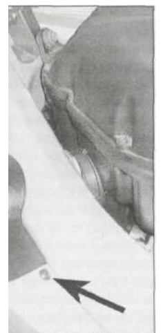
3.7 Each intake duct cover is secured by three screws (arrowed)
