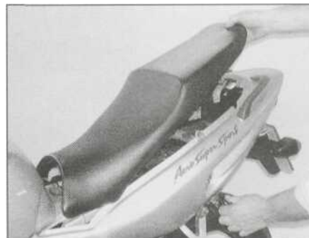
2.1 On YZF models, turn the key to release the latch and lift the rear of the seat
