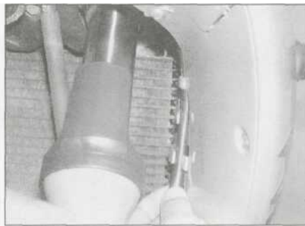
3.19 Free the speedometer cable from its guides
