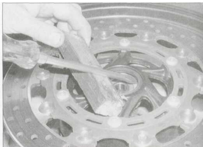
16.3 Lever out the grease seal
