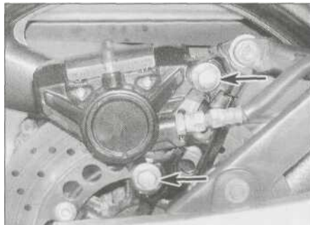
7.3a Unscrew the bolts (arrowed)...
