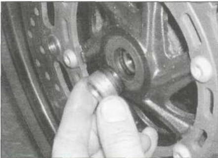
14.6a Remove the spacer ...
