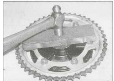
16.31 Press or drive the seal into the coupling - using a piece of wood as shown sets the seal flush with the rim
