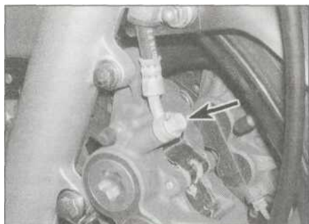
3.2 Unscrew the brake hose banjo bolt (arrowed), noting its alignment - YZF model
