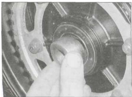
15.7a Remove the plain collar from the left-hand side ..
