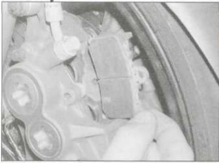
2.2a Lift the pads out of the caliper .. .
