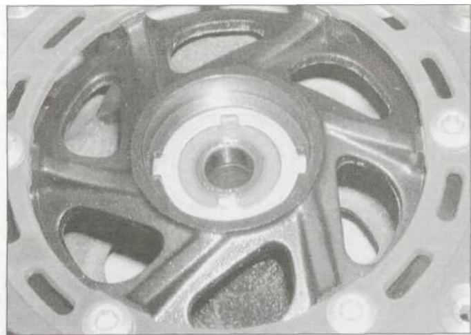
16.12 Fit the drive plate
