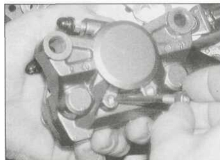
6.2c Remove the pad pins ...
