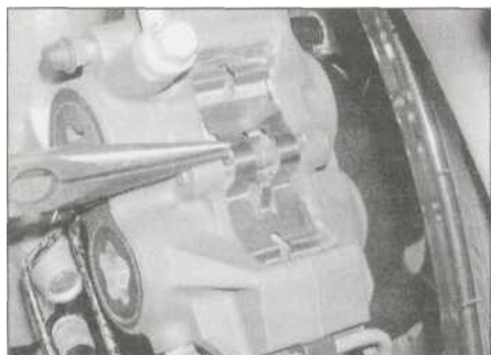
2.1 a Remove the retaining clips
