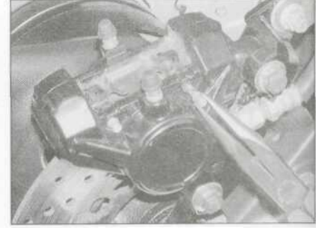
6.1 c Withdraw the pad pins .
