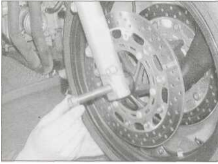
14.11b ... and insert the axle
