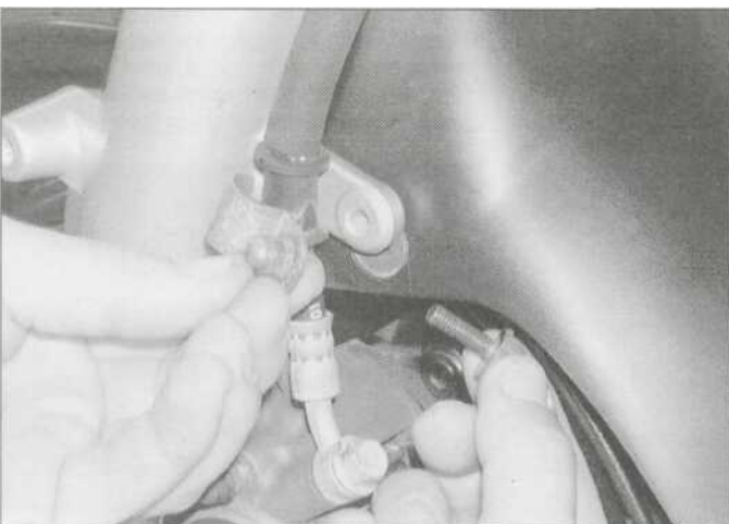
3.1 a On YZF models, unscrew the nut and withdraw the bolt to free the hose from its clamp
