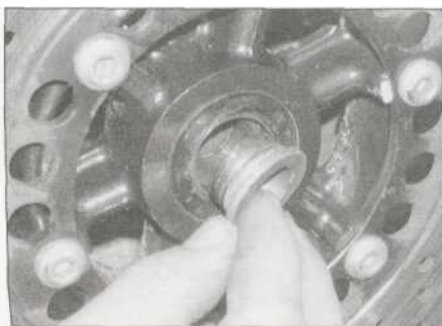
15.7b ... and the shouldered collar from the right-hand side
