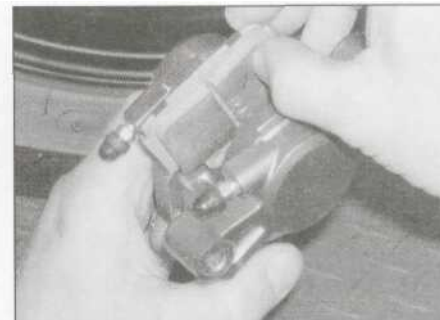
6.2d ... and withdraw the pads
