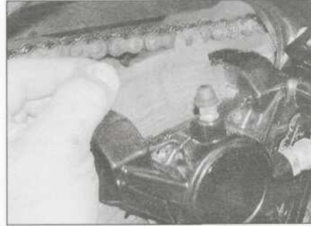
6.1e Lift out the pads ...
