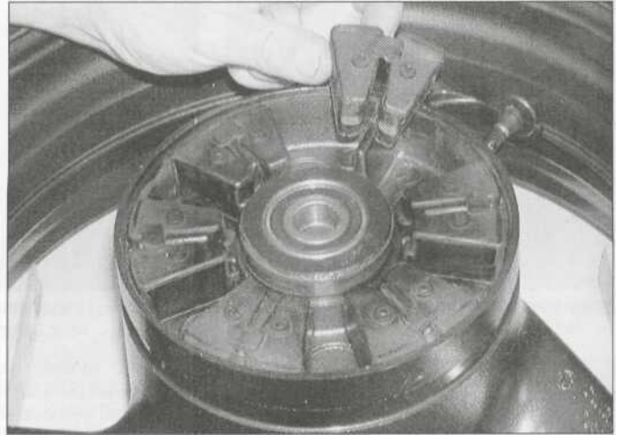
16.15b ... and remove the rubber damper segments
