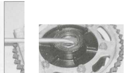
16.26c Lever out the grease seal
