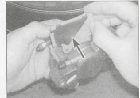
6.2e Remove the shim (arrowed) from the back of the pad, if one is fitted
