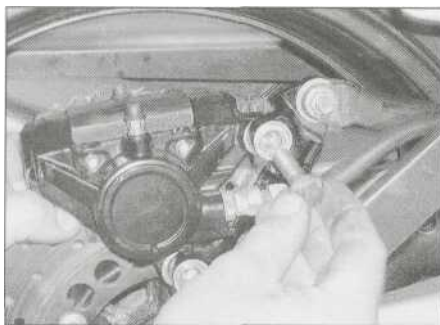
7.15a Install the caliper bolts ...
