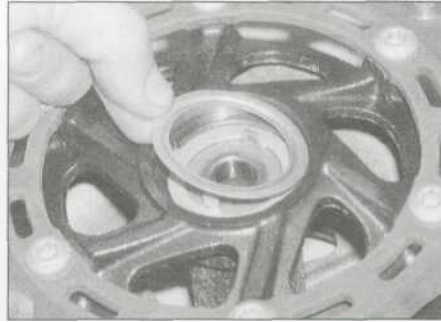
16.4b ... then lever out the retainer plate...
