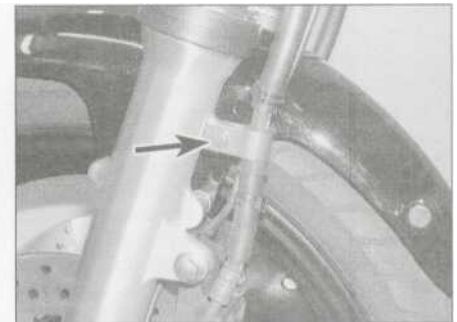
6.2b On FZS models, unscrew the bolt (arrowed)
