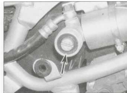
12.9 Compression damping adjuster (arrowed)
