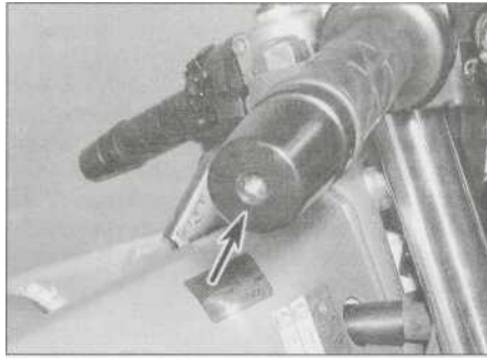
5.5 Unscrew the end-weight (arrowed) if required
