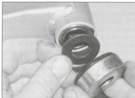
14.2a Remove the cap with its seal, and the washer..
