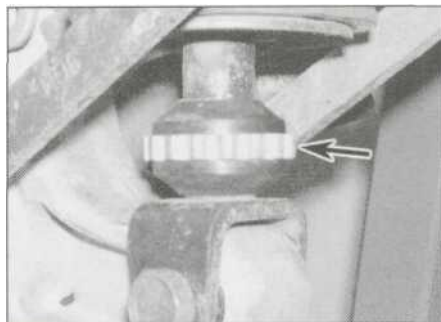
12.8 Rebound damping (arrowed) adjuster
