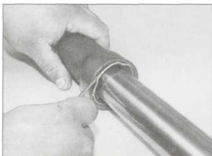
7.11 Prise out the retaining clip using a flat-bladed screwdriver
