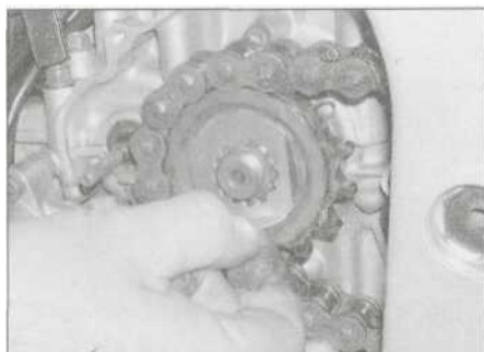
16.10a Fit the new lockwasher ...
