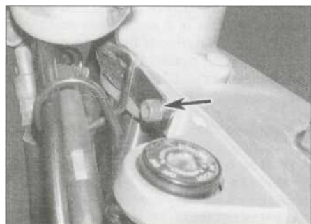
8.3c Unscrew the bolt (arrowed) and displace the cable guide
