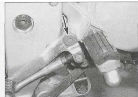
3.8b Unscrew the pivot bolt (arrowed) and remove the lever, noting the washers
