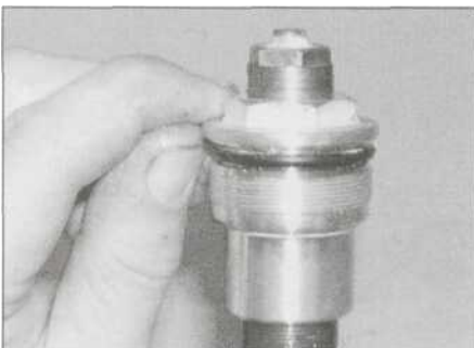
7.28a Fit a new O-ring onto the top bolt
