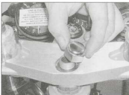
8.14b ... and the steering stem nut...
