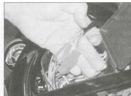
8.4b Disconnect the ignition switch wiring connectors
