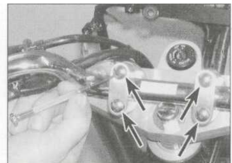
5.8 Remove the blanking caps, then unscrew the bolts (arrowed)
