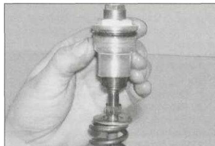
7.28b Thread the pre-load adjuster and top bolt assembly onto the damper rod and tighten it against the locknut
