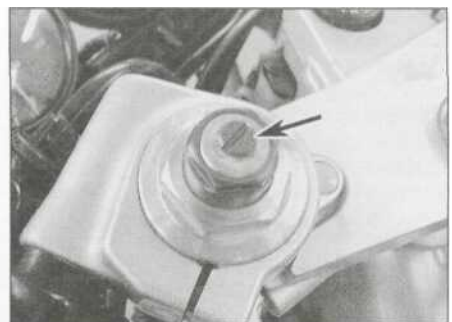
12.3 Rebound damping adjuster (arrowed)
