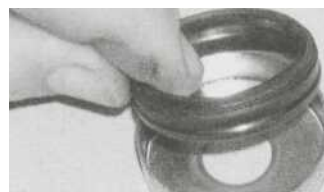
14.2c Check the seals and renew them if necessary
