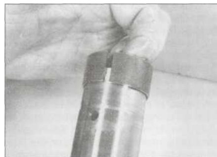
7.18 Prise the bottom bush apart using a flat-bladed screwdriver and slide it off
