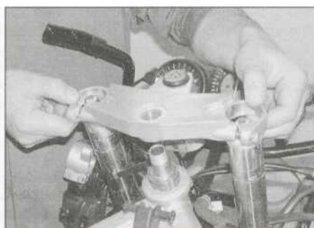
8.6b Ease the top yoke up off the steering stem
