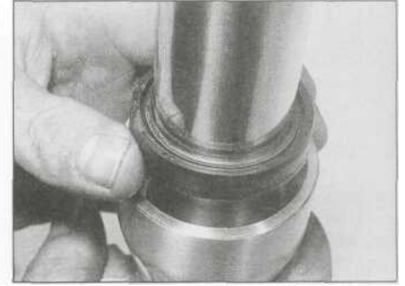
7.23 Make sure the oil seal is the correct way up
