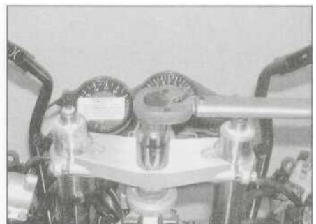
8.14c ... and tighten it to the specified torque
