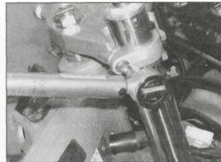
6.9c ... and the top yoke clamp bolt to the specified torque settings
