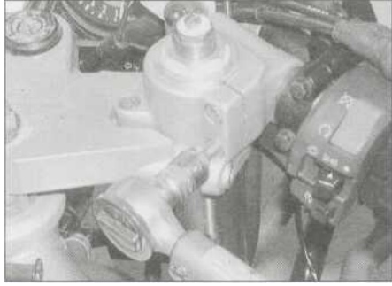
5.9a Tighten the various bolts to the specified torque settings
