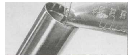
7.26a Pour the oil into the top of the tube
