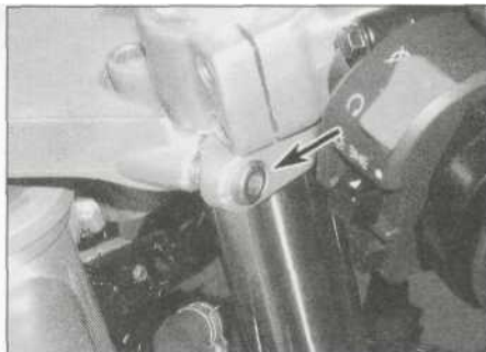
6.6a Slacken the fork clamp bolt (arrowed) - YZF model
