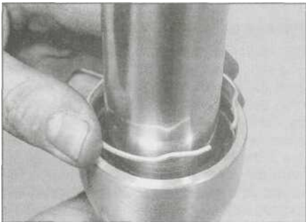
7.24 Install the retaining clip ...
