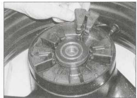
17.3 ... and remove the rubber dampers
