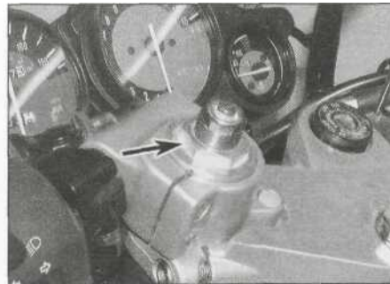
6.6b Slacken the top bolt (arrowed) if the forks are to be disassembled
