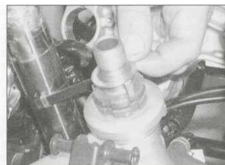
8.7a Remove the tabbed lockwasher ...
