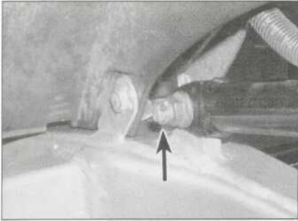
13.2b Remove the split pin (arrowed), then unscrew the nut..
