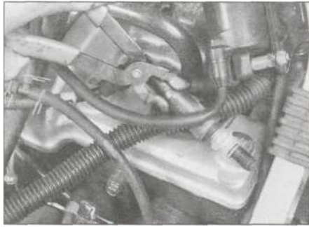
2.2 Ground (earth) the spark plug and operate the starter - bright blue sparks should be visible
