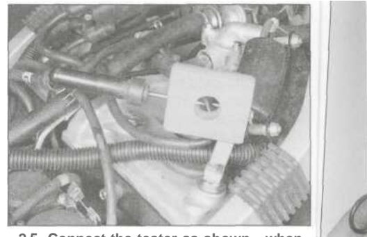
2.5 Connect the tester as shown - when the starter is operated sparks should jump between the nails
