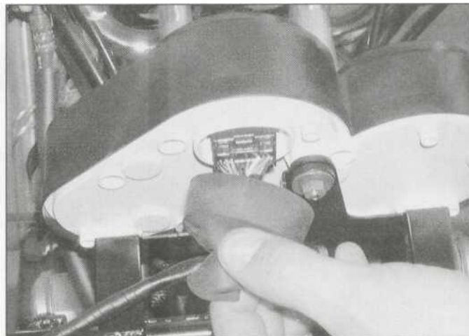
15.13 Disconnect the wiring connector from the instrument cluster
