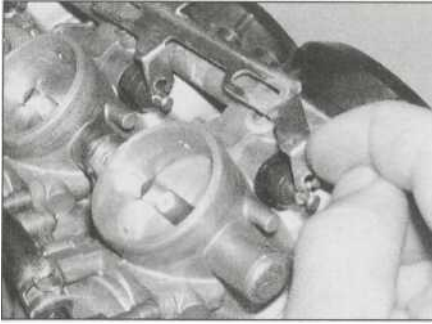
8.12c Remove the linkage bar, noting how the arms locate on the plungers ...
