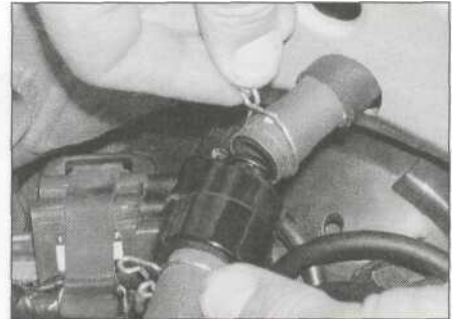
7.7b Detach the air vent hose at the union
