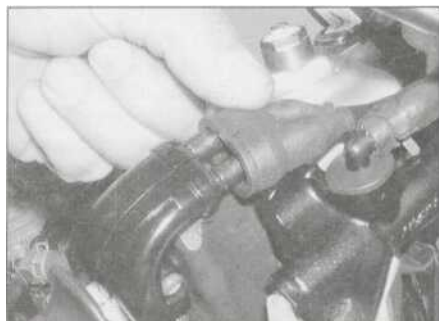
11.4a Pull the boot back off the housing ..
