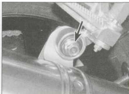
13.3 ... and remove the mounting bolt (arrowed)
