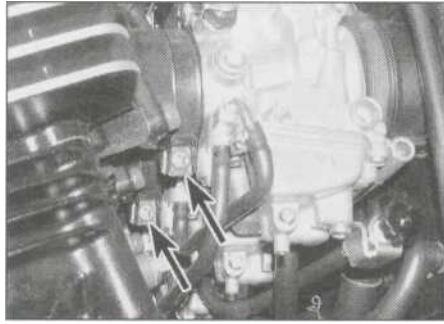
7.11c Clamp screws (arrowed)- FZS models
