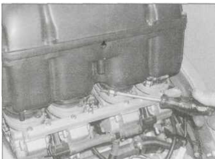
4.3c ... and the four carburettor clamp screws
