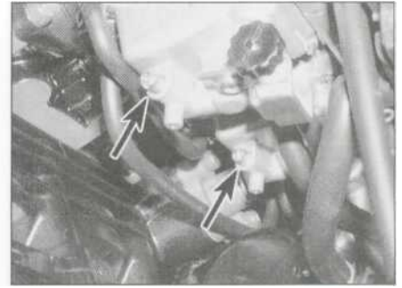
7.12 Carburettor drain screws (arrowed) - FZS models
