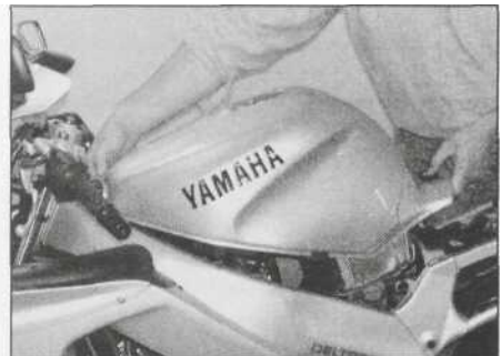
2.5b ... and remove the tank
