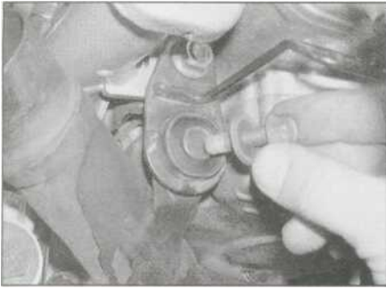
13.10a Downpipe assembly bolt - YZF models
