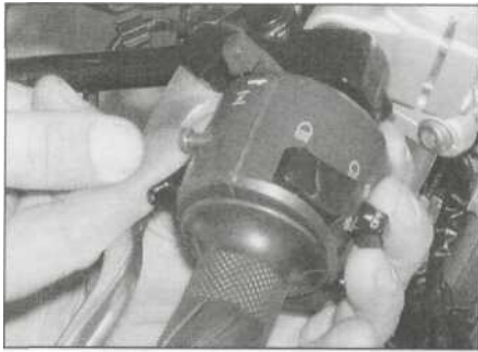
12.3a Remove the housing screws ,
