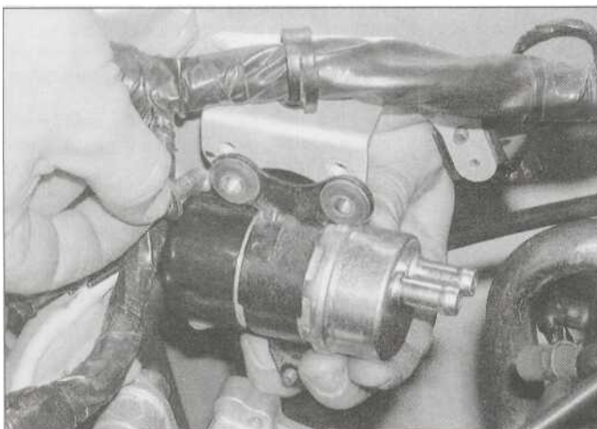
14.9b ... then unscrew the bolts and remove the pump
