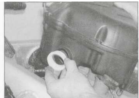
4.4b ... and remove the collars, if required
