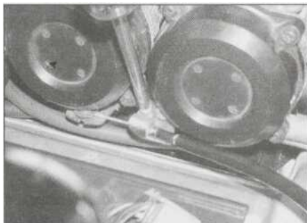
7.4a Slacken the clamp screw ...
