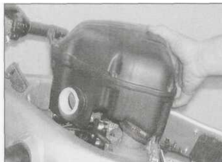
4.4a Lift the housing off the carburettors..
