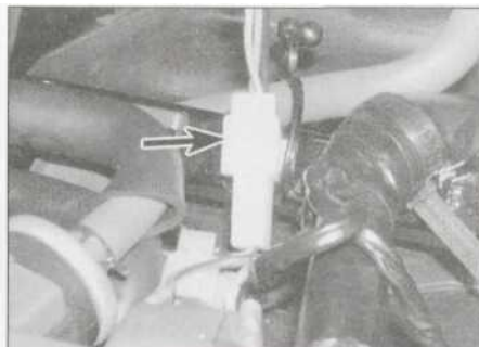
2,10b ... and disconnect the wiring connector
