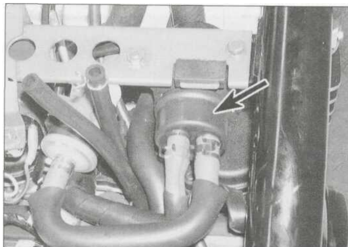
14.1c Fuel pump (arrowed) - FZS models
