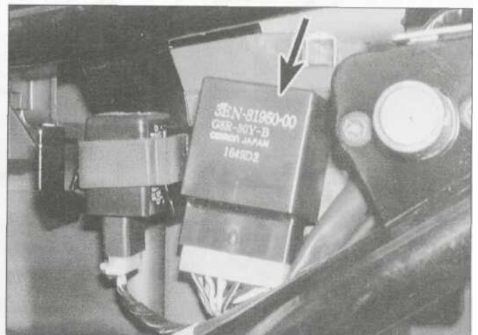
14.1d Relay (arrowed) • FZS models
