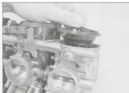
8.3b ... then carefully remove the diaphragm/piston assembly
