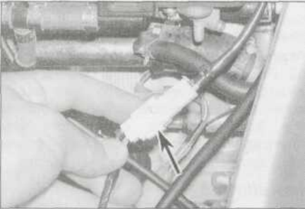
7.8a On YZF models, disconnect the throttle position sensor wiring connector (arrowed)
