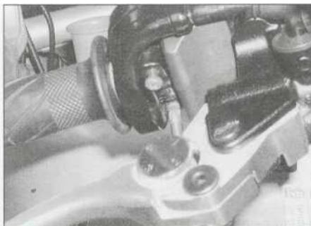
11.4b ... and remove the housing screws
