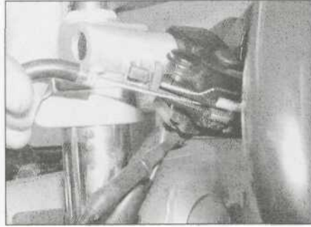
18.6a Align the slots and slip the cable out of the bracket...
