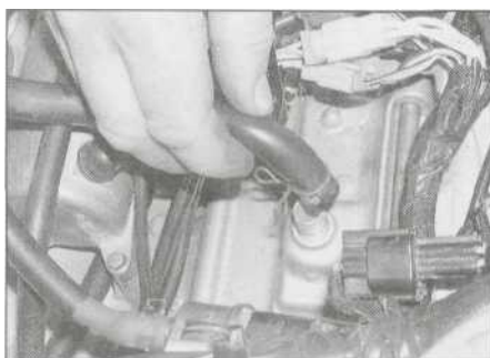
5.19 Detach and remove the crankcase breather hose if required
