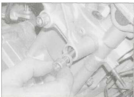
5.23 Do not forget the washers with the right-hand front bolts
