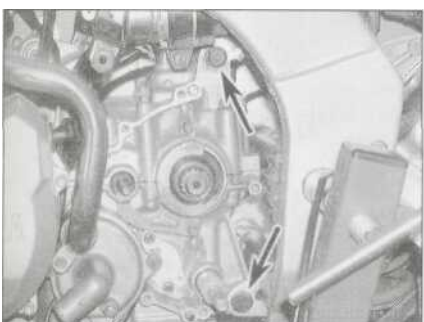
5.21 e Withdraw the bolts (arrowed) from the left
