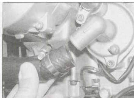
5.7b Slacken the clamps and detach the hoses from the water pump ...
