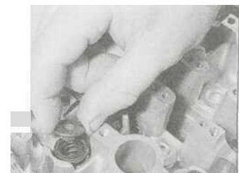
13.26c ... then fit the spring retainer
