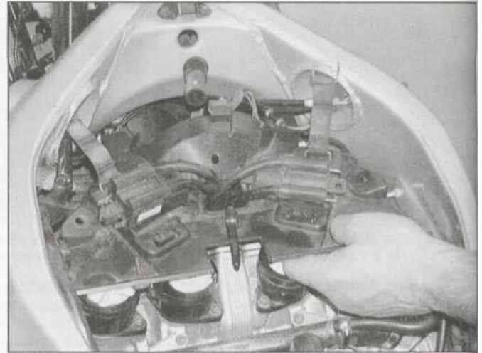
8.1 b Remove the coil mounting plate, noting how it fits
