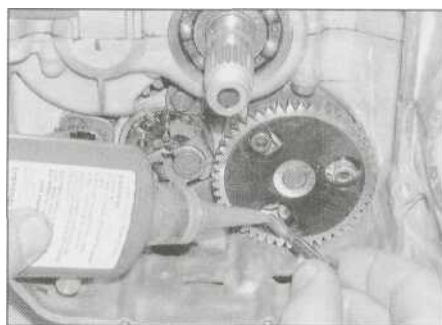
21.14d Apply a suitable non-permanent thread locking compound to the mounting bolts
