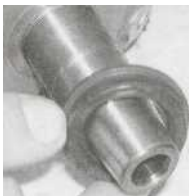
28.2b Remove the oil seal and discard it
