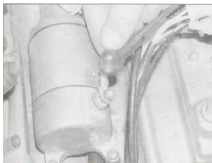
5.17 Unscrew the nut and detach the starter motor lead from the relay
