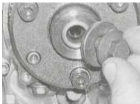
19.5 Unscrew the bolt and remove the washer
