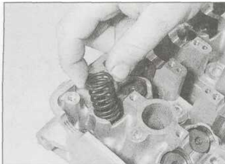
13.26b Fit the valve spring with its closer-wound coils facing down ...
