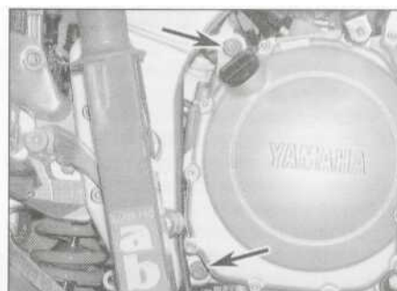
5.21 d Remove the nuts (arrowed) from the rear mounting bolts
