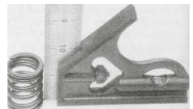
13.17b Check the valve springs for squareness
