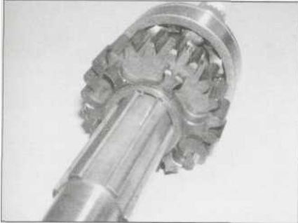
30.16d ... making sure it locates correctly in the groove
