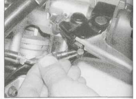
18.6b ... and the nipple from the lever
