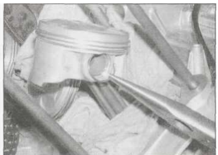
15.17 Do not over-compress the circlips when fitting them into the piston
