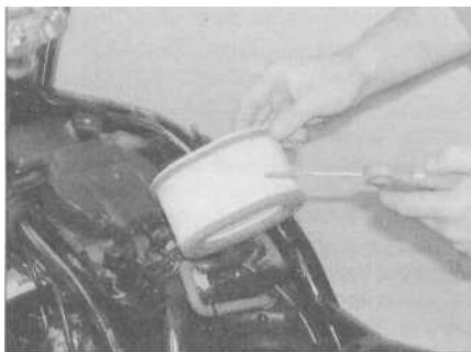
5.4 Clean the element using compressed air if available
