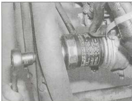
21.3a Unscrew the filter ...
