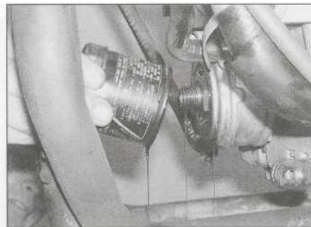
21.3b ... and drain the oil into the tray
