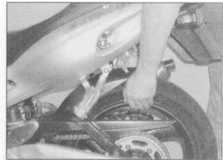
19.7b Checking for play in the suspension linkage bearings
