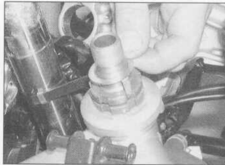
20.8a Remove the tabbed lockwasher.
