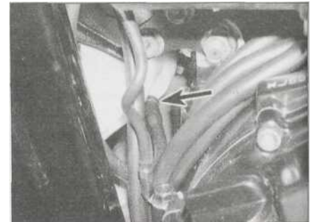
22.4b Coolant reservoir hose • FZS models
