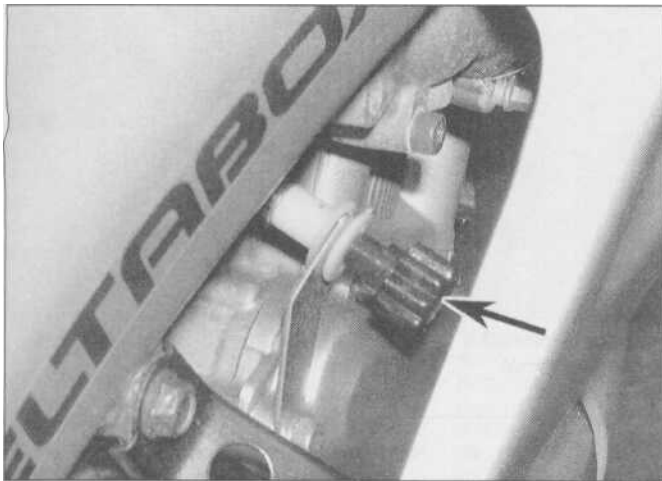
3.3a Idle speed adjuster screw (arrowed) - YZF models
