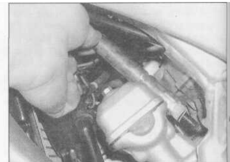
2.8 Thread the plug as far as possible turning the tool by hand
