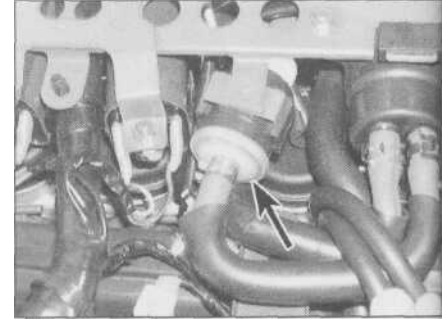
6.8b In-line fuel filter (arrowed) - FZS models
