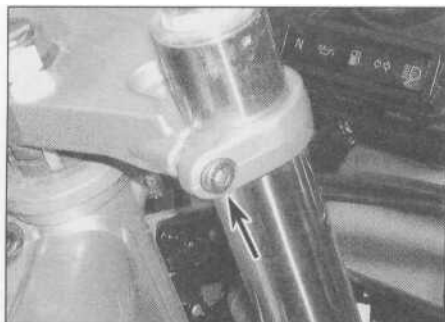
20.6a Slacken the fork clamp bolt (arrowed) on each side ...
