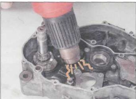
2.15 Using heat to free a seized fastener
