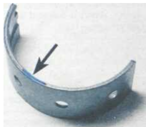
5.14 Shell bearings are either plain or grooved. They are usually identified by colour code (arrow)
