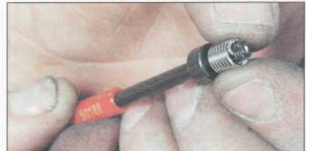
2.28 ... fit insert on the installing tool...
