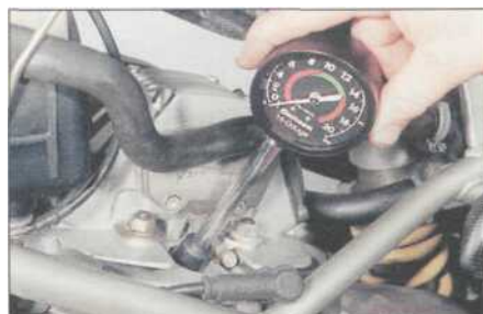
3.20 Using a rubber-cone type cylinder compression gauge
