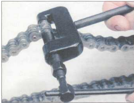
8.8 Assemble the chain riveting tool over one pin at a time and tighten it fully
