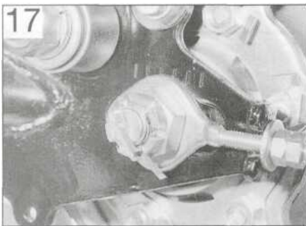
Castellated type wheel axle (spindle) nut must be secured by a split pin or R-pin
