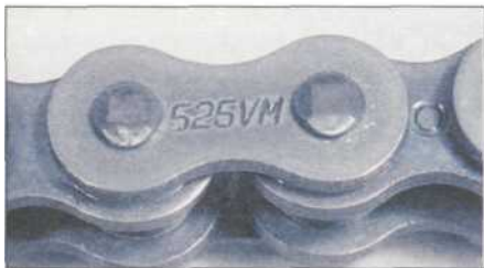
8.10 Typical chain size and type marking
