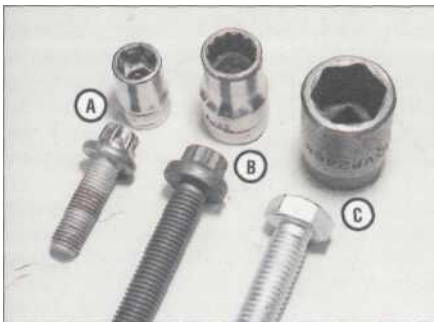
2.2 External Torx (A), splined (B) and hexagon (C) fasteners, with corresponding sockets
