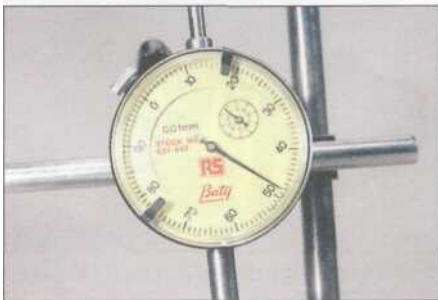
3.17 Dial gauge reading of 1.48 mm
