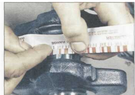
3.16 Measuring the width of the crushed Plastigauge
