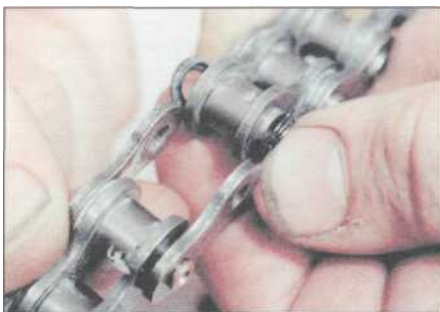
8.3 ... and separate the chain link
