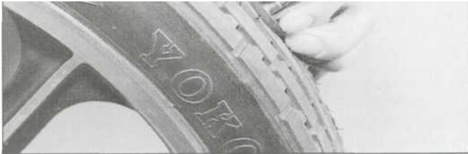
Checking the tyre tread depth
