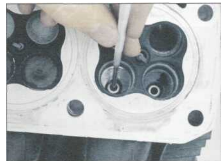
3.9 Expand the small hole gauge in the bore, lock its position ...
