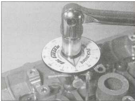
Angle-tightening cylinder head bolts
