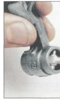
3.7 Expand the telescoping gauge in the bore, lock its position ...
