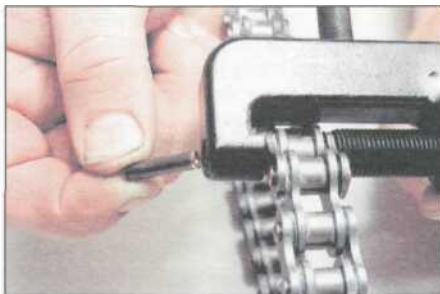
8.2 ... withdraw the pin, remove the tool...
