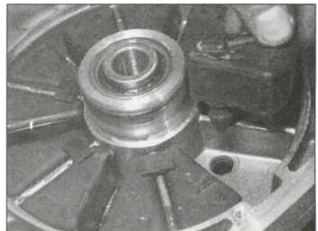
Cush drive rubbers dampen out transmission shocks
