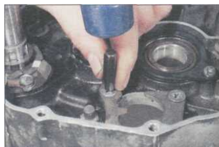
2.13 A sharp tap on the head of a fastener will often break free a corroded thread
