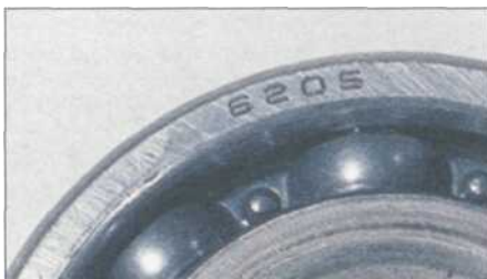
5.16 Typical bearing marking
