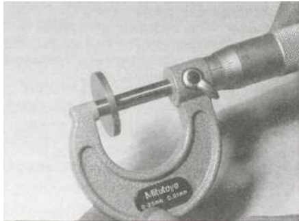
Tappet shims are measured with a micrometer
