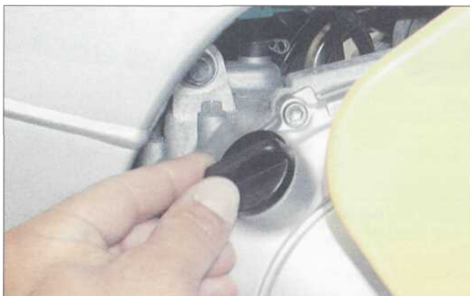
3 If the level is below the minimum line, remove the filler cap from the top of the clutch cover.
