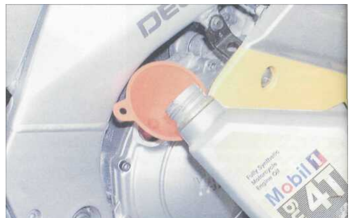
4 Top the engine up with the recommended grade and type of oil, to bring the level up to the maximum level on the window.
