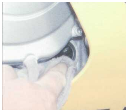
1 Wipe the oil level inspection window, located on the right-hand side of the engine, so that it is clean.
